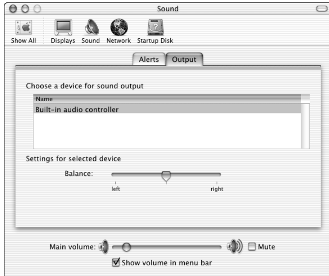
Figure 15-28: Choose an audio output device and set its stereo balance by clicking the Output tab in Sound Preferences.
