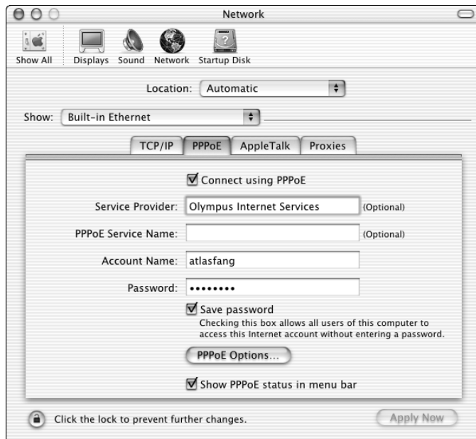
Figure 18-8: PPPoE settings are required by some DSL and cable modem Internet providers.
