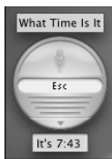
Figure 17-8: Help tags above and below the speech feedback window display the command that the computer recognized and its response, if any.
