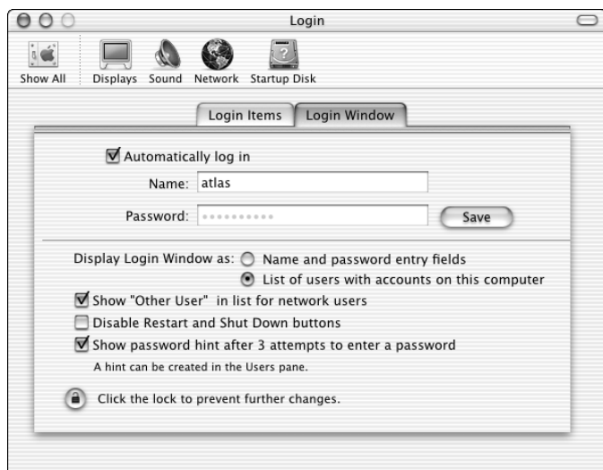
Figure 16-7: Click the Login Window tab of Login Preferences to set automatic login on or off and to set other login options.
