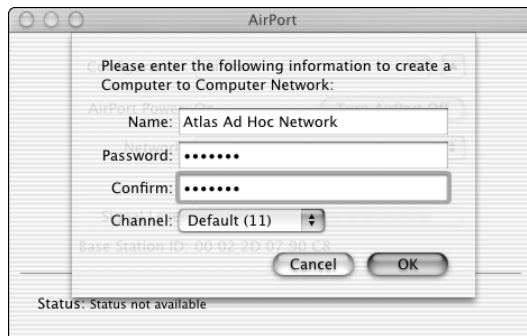
Figure 18-1: Create an ad hoc wireless network from any Mac with an AirPort card.
