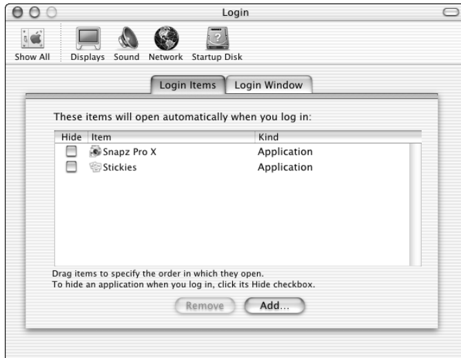
Figure 16-8: Click the Login Items tab in Login Preferences to change the list of items that open automatically when the current user logs in.
