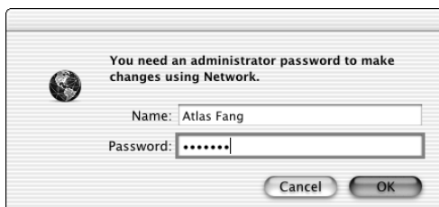
Figure 15-3: Unlock protected preference settings by entering the name and password of an administrator account.
