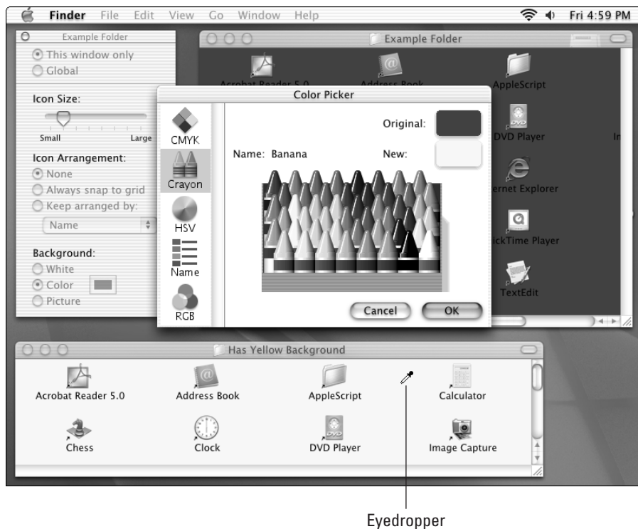
Figure 4-6: Set a background color in the Color Picker. (Press Option to make the pointer an eyedropper for picking up any displayed color.)
