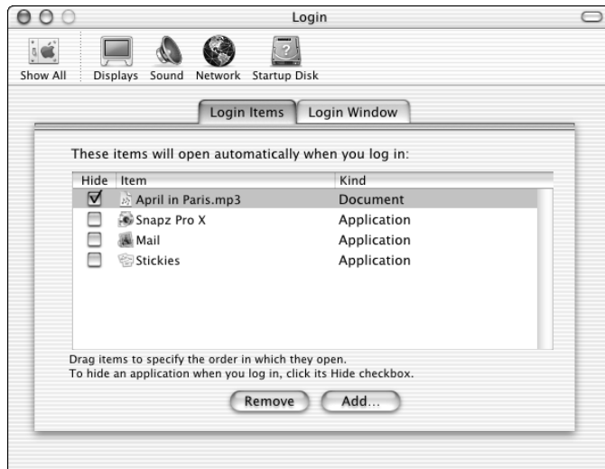
Figure 15-34: Set up a list of items opened during login by clicking the Login Items tab of Login Preferences.
