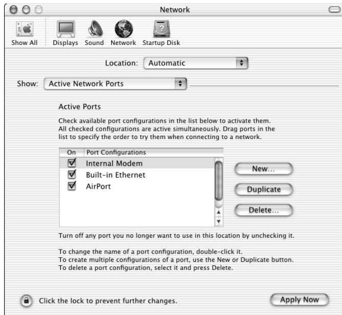
Figure 18-14: Change the Active Network Ports settings in Network Preferences to affect which port configuration Mac OS X uses.
