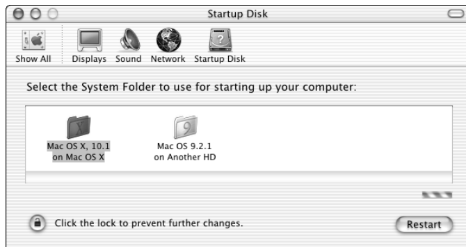
Figure 15-33: Startup Disk Preferences specifies which Mac OS System Folder is used the next time your computer starts up.
