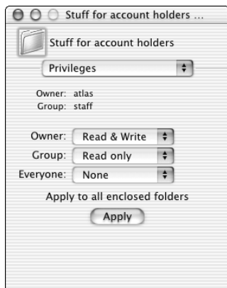
Figure 19-2: Each of your files and folders can have different privilege levels in three user categories.
