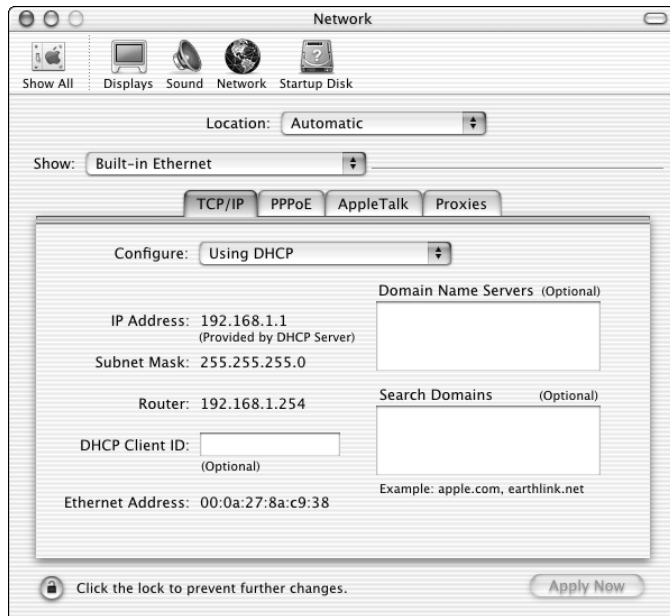
Figure 18-3: Configure network settings in Network Preferences (the Network pane of System Preferences).
