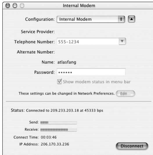
Figure 6-2: Internet Connect displays information about an active modem connection at the bottom of the connection window.
