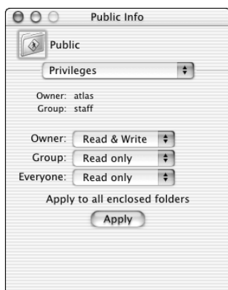
Figure 16-9: Change privilege settings for a folder or file in the Finder's Info window.
