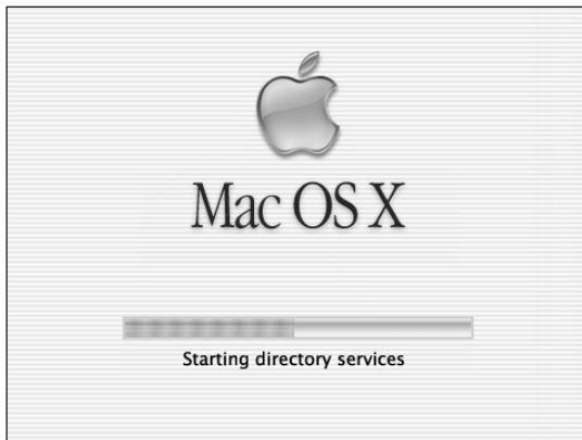
Figure 2-1: A progress gauge and a series of messages report on the startup process.
