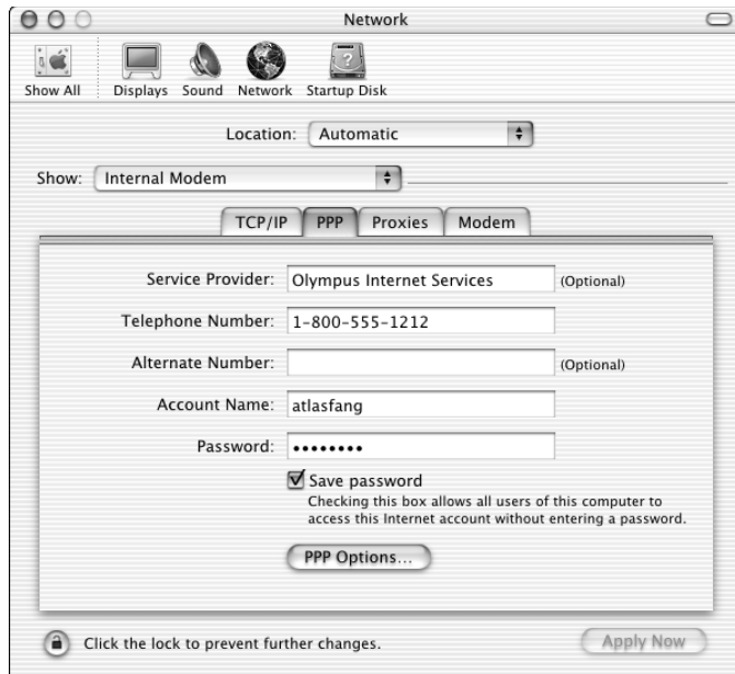
Figure 18-11: PPP settings specify the contact and account information for a modem or ISDN connection to the Internet or a remote network.
