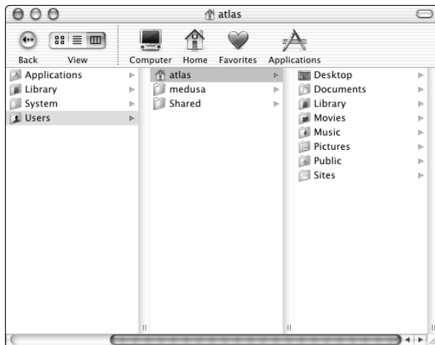
Figure 1-5: The Finder's column view shows several levels of folder hierarchy at a glance.
